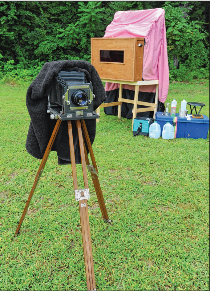
Terri Cappucci’s set-up for working in the wet plate collodion process includes, here, a 1930s 5x7 Vageeswari field camera (she also works with a 4x5 Graflex camera), her hand-built “dark box” and an array of chemicals for sensitizing and processing the aluminum plates. Cappucci is very careful about storage, use and disposal of all chemicals.
