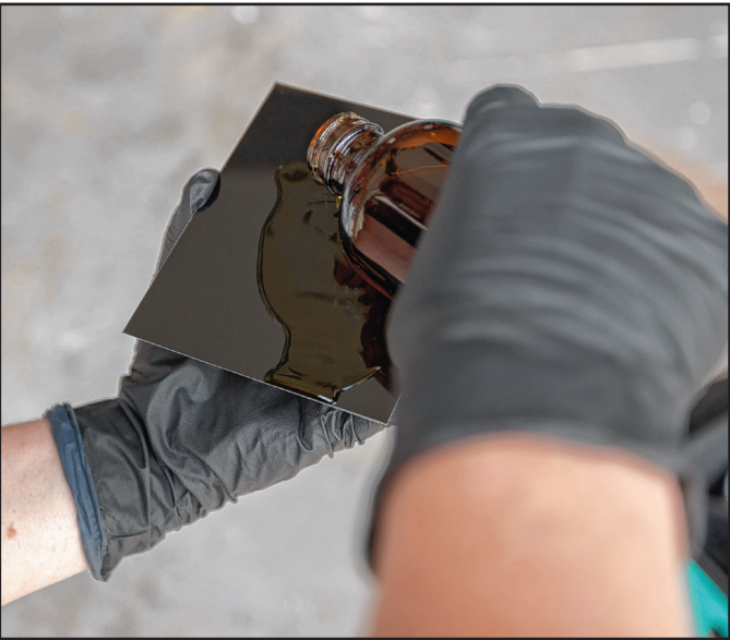
Cappucci pours the collodion over the aluminum plate to coat it, creating a base for the silver nitrate to adhere to. Once the collodion becomes tacky, Cappucci will sensitize the plate in silver nitrate. From this point, the plate goes directly into a plate holder while it’s still wet and then into the camera, where the image is exposed.
